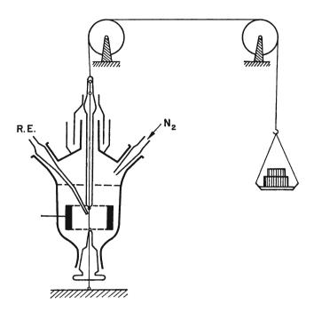
A sketch drawn by V. S. Bagotsky: the cell for electrochemical measurements on a wire under mechanical load (stretching)
